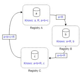
Figure 5. Example algorithm for MPC.
