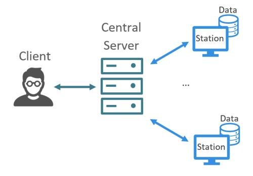
Figure 2. High level IT architecture of vantage6. The arrows denote communication between components over the internet. Image adapted from (1)
